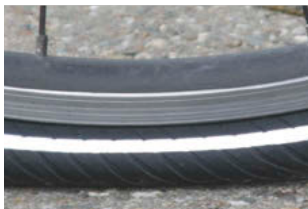
Illustration 82 : Pression largement insuffisante
