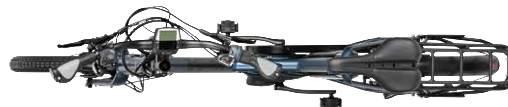
Here, i:SY with handlebars twisted 90° (SPEED LIFTER Twist T22 fitted as standard) and pedals retracted (folding pedals fitted as standard)
