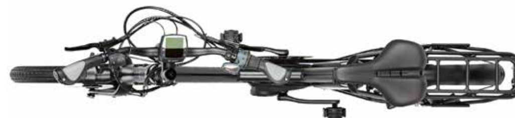
Here, i:SY with handlebars twisted 90° (SPEED LIFTER Twist T22 fitted as standard) and pedals retracted (folding pedals fitted as standard)
