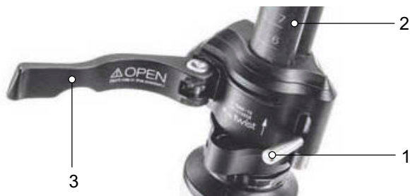
Figure 91: Opened clamping lever on the stem quick release (3) on the stem (2), version I, with locking lever on the stem (1)
