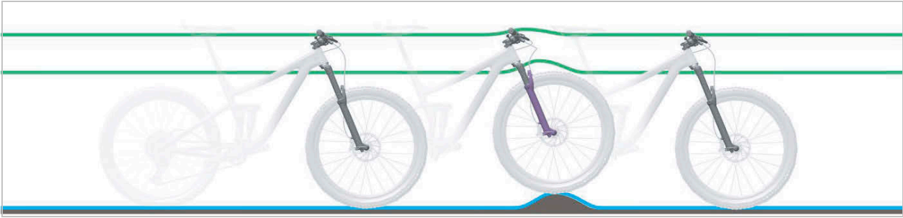
Figure 17: Optimum suspension fork ride performance over bumps
