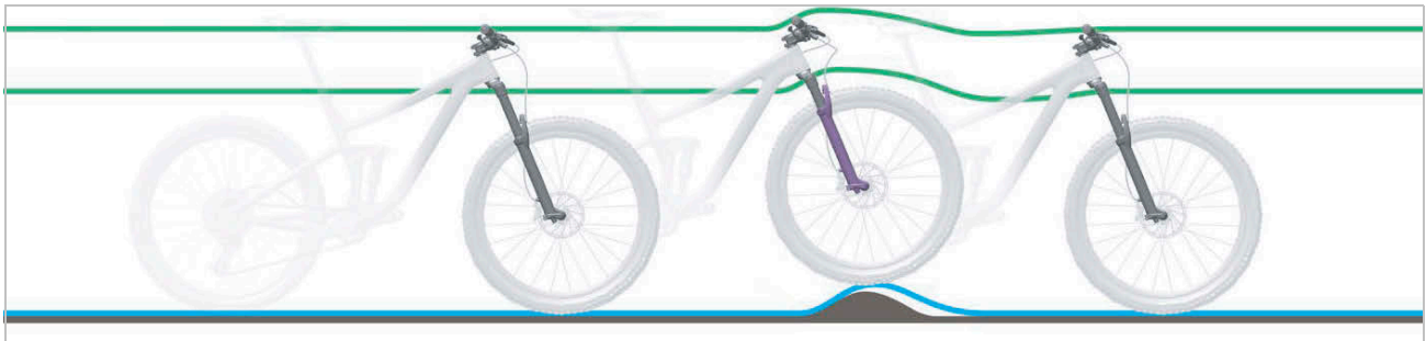
Figure 222: Excessively hard damping in the suspension fork on bumps
