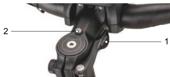
Figure 92: Stem, version II with clamping lever on the stem quick release (1) and unlocking knob (2)
